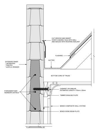
NOTE: THIS IS A PRELIMINARY DESIGN THAT HAS NOT BEEN APPROVED BY A STRUCTURAL ENGINEER. ESTIMATED MAXIMUM OF 3 COARSES TO BE REINFORCED AND CORE FILLED.
