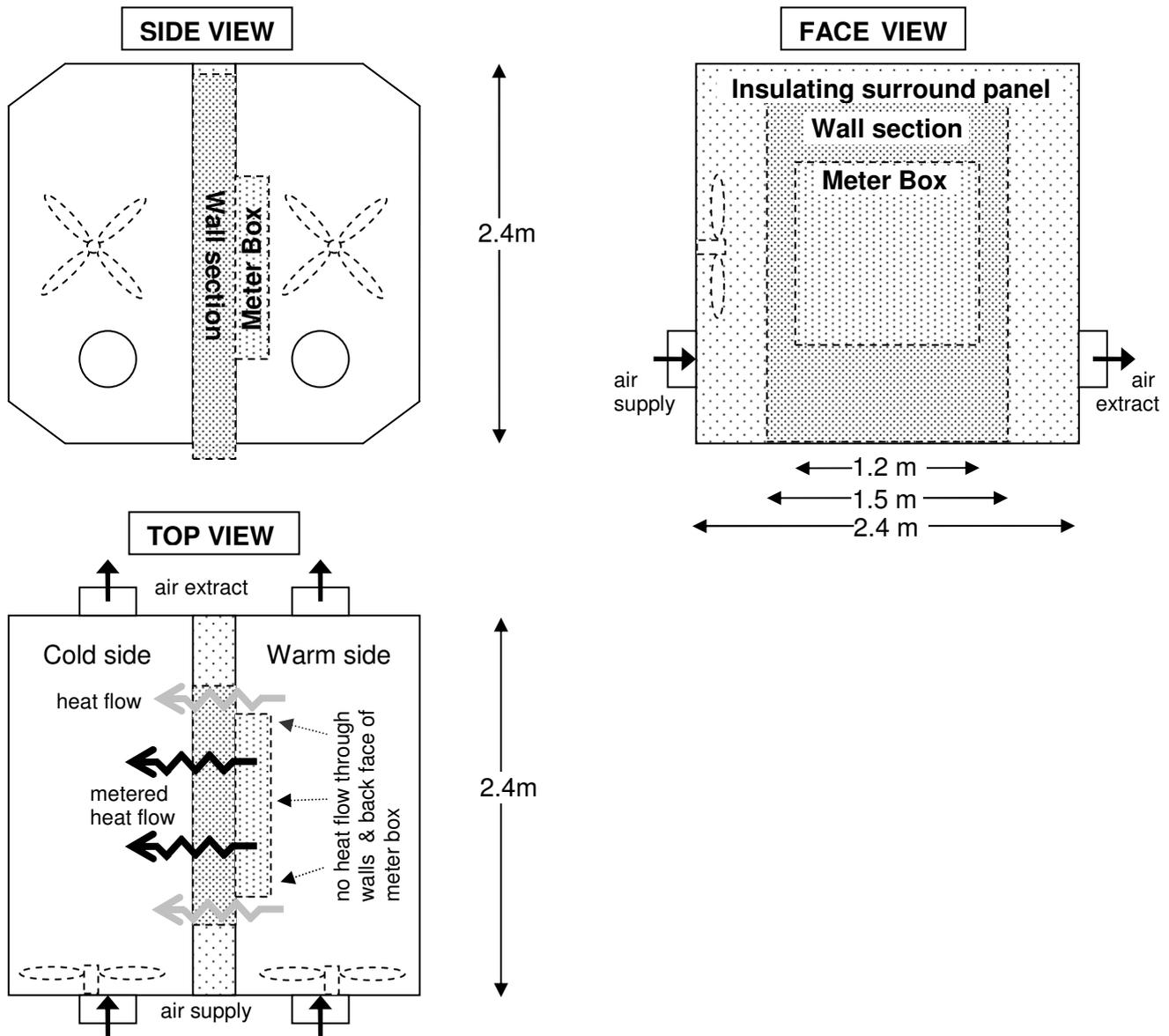
Figure 4. Schematics of Guarded Hot Box Apparatus
