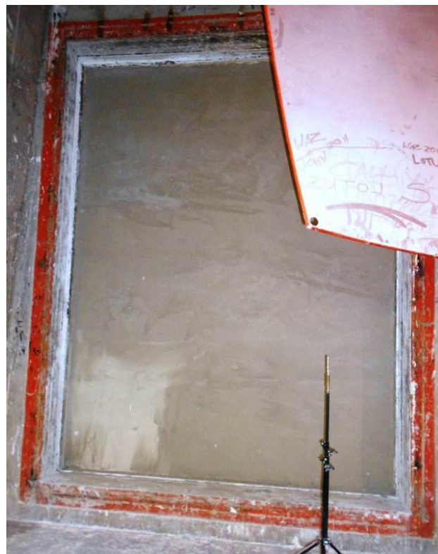
Figure 3: 226mm Footprint Rendered 35mm Benex Panel Wall System built into the Test Aperture for testing as seen from the Receive Room.
