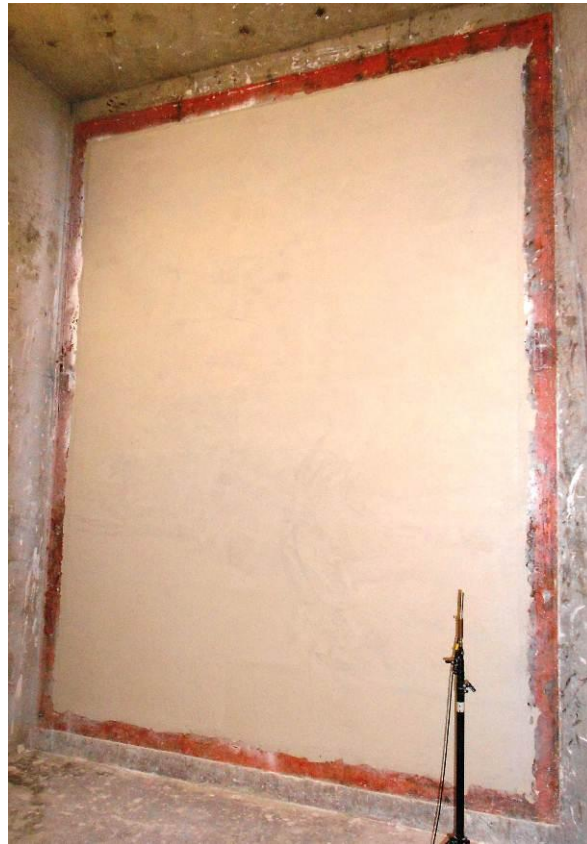
Figure 3: 226mm Footprint Rendered 35mm Benex Panel Wall System built into the Test Aperture for testing as seen from the Receive Room.
