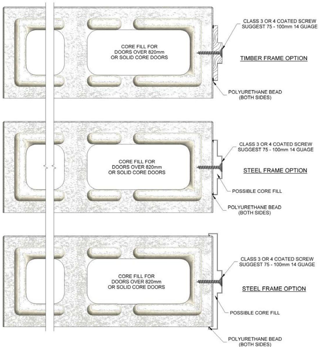
A variety of timber and steel door jambs can be fitted directly to a Benex block wall. As noted in the diagram above, the steel jamb can be core filled if required.
