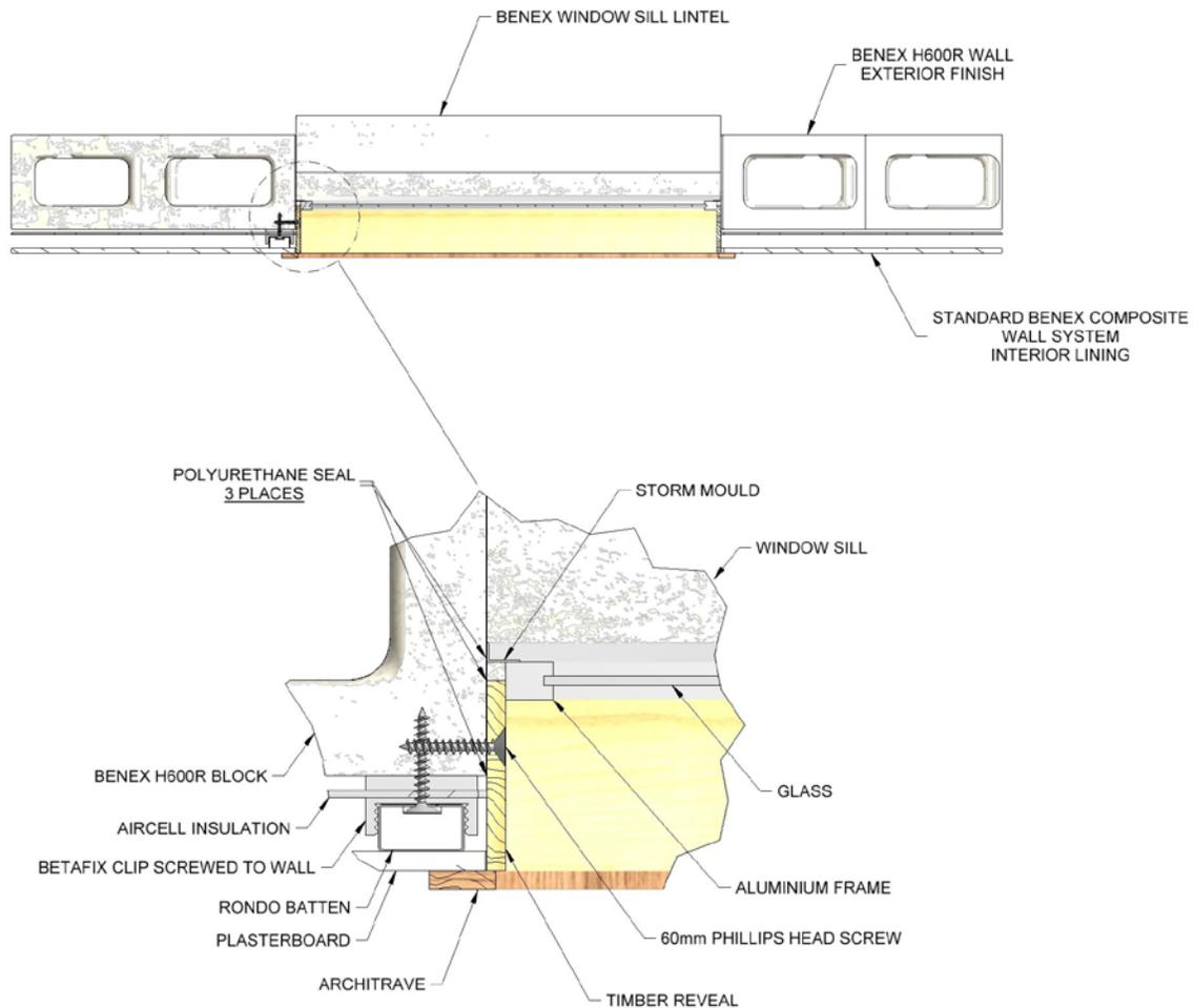
When installing windows or door frames in a Benex wall, firstly determine the position of the window or door and mark the area out on the slab in the case of a door, or one course lower than the sill in the case of the window.
