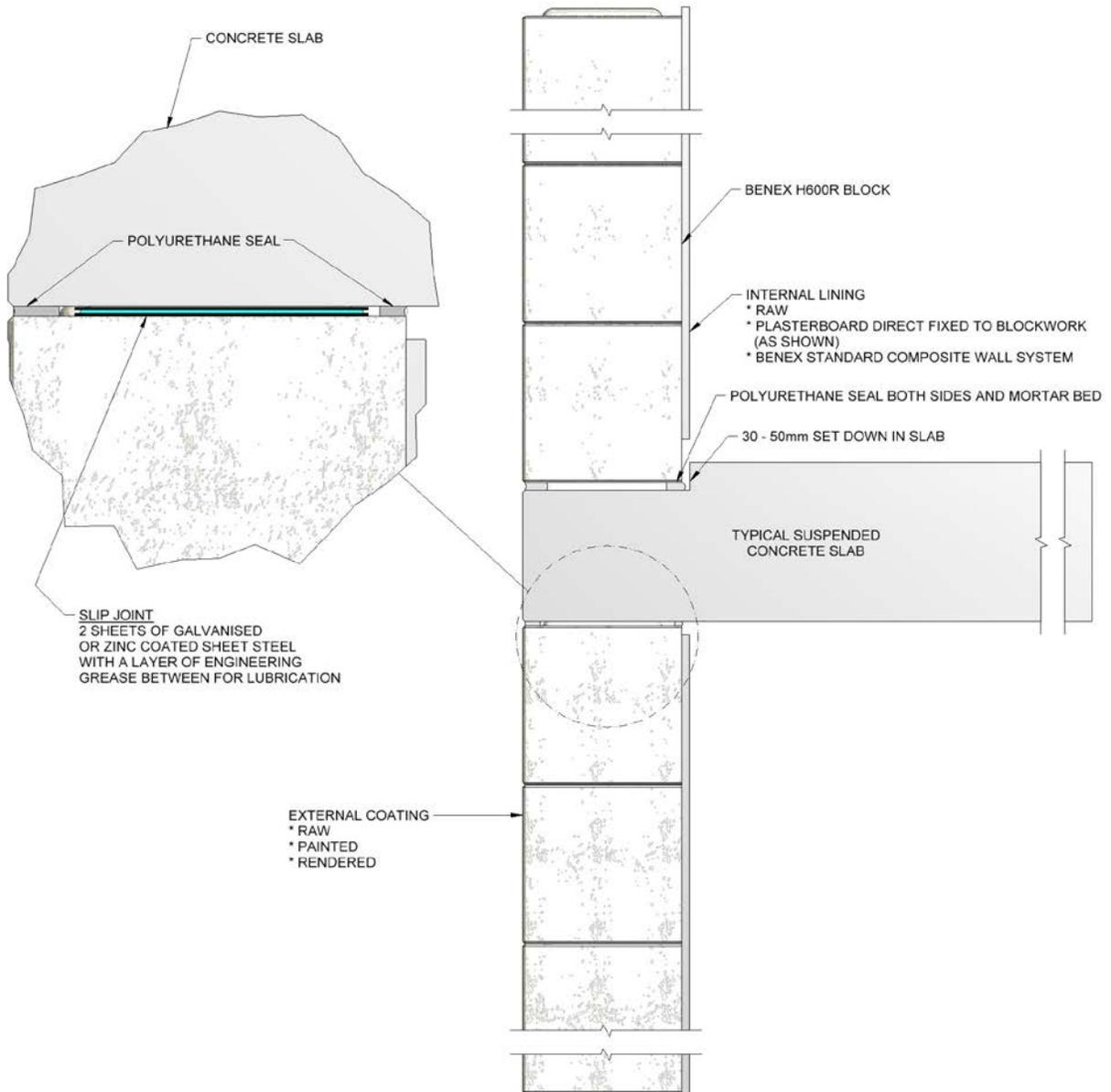
Walls supporting suspended concrete floors require a suitable slip joint at the interface.
