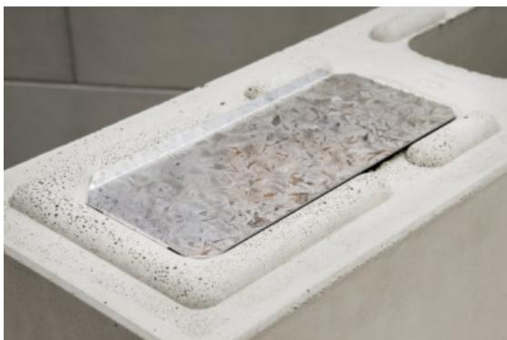
The Benex bond beam plates allow Benex installation crews to install a bond beam wherever they need to. They also eliminate the need for different types of blocks on site, thus saving confusion at the ordering stage and making for a very simple but effective solution.
