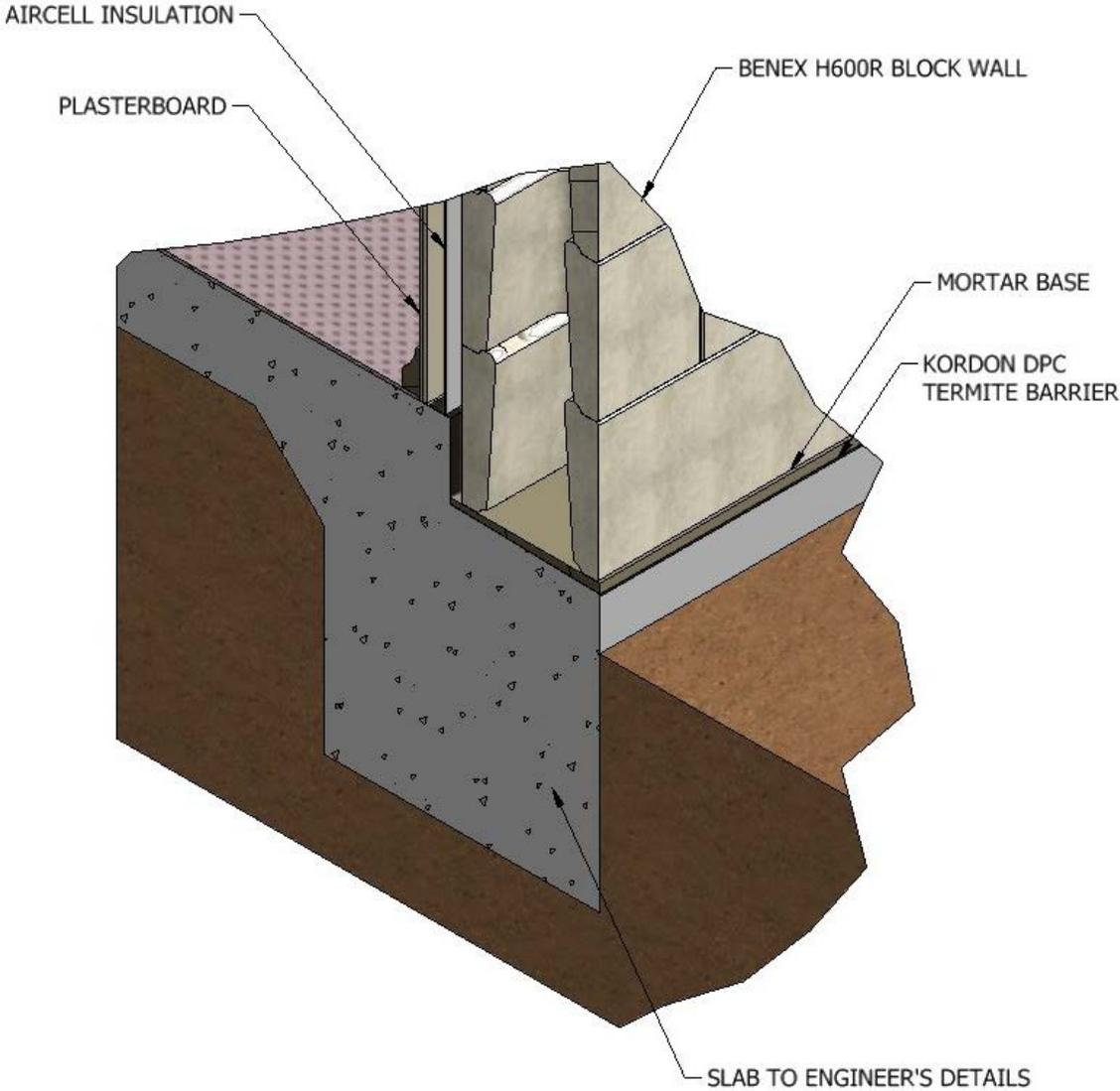
A slip join/bond breaker (DPC) must be installed between the first course and the footing or slab on all internal and external walls to allow for differential movement between the blocks and the support structure.
