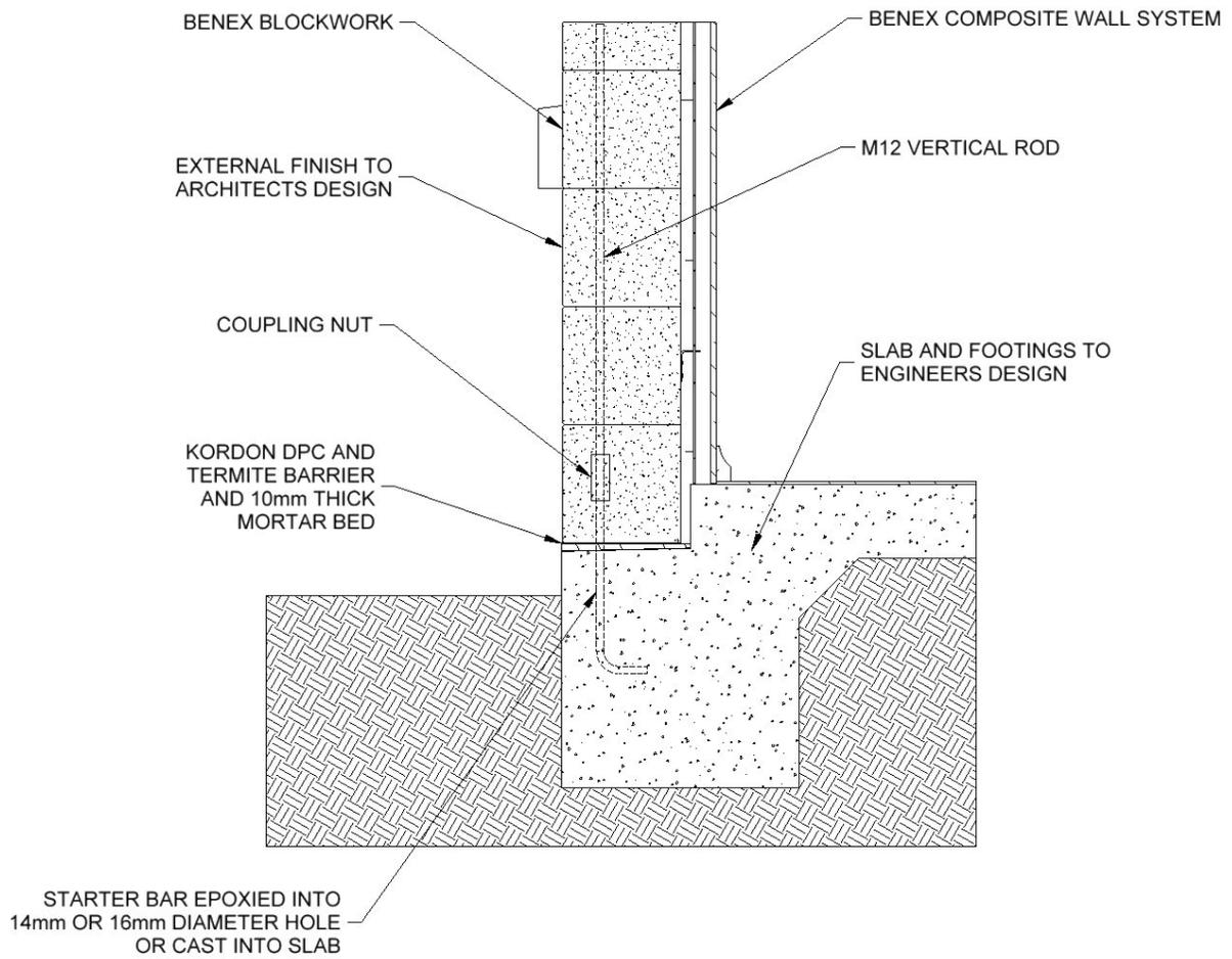
CORE FILLED BLOCKWORK ONLY REQUIRED WHEN SPECIFIED BY STRUCTURAL ENGINEER
